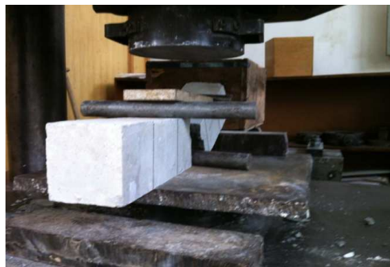
Figure 2 Beam at failure
