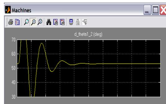
3) We present the changes of angle  $\delta_{12}$  in the case of short circuit single-phase and three phase:
