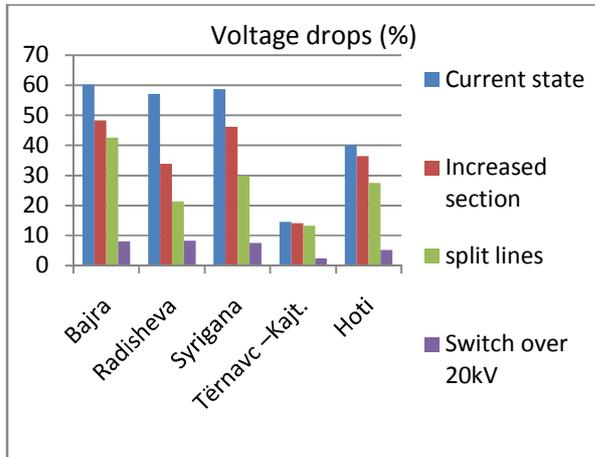
**Figure 2 Comparison of voltage decrease in line J01**
