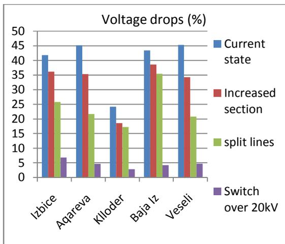
**Figure 3 Comparison of voltage decrease in line J02**
