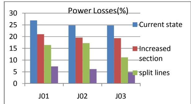
**Figure 1 Comparison of energy losses for three lines**
