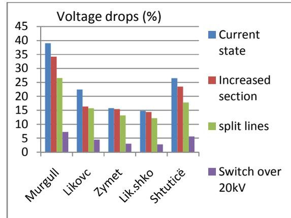
**Figure 4 Comparison of voltage decrease in line J03**
