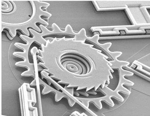
**Figure 2 MEMS Device (Micro machine).**
