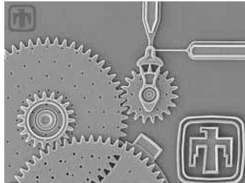
**Figure 3 Micro gear using MEMS**
