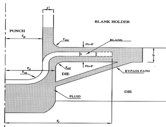
**Figure 1 hydro assisted deep drawing process**
