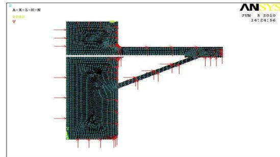
**Figure 2 Boundary Conditions of Hydro Assisted Deep Drawing Model**
