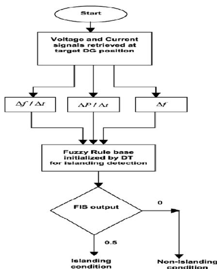
Figure 4 Flowchart for the proposed fuzzy rule-based scheme for islanding detection
