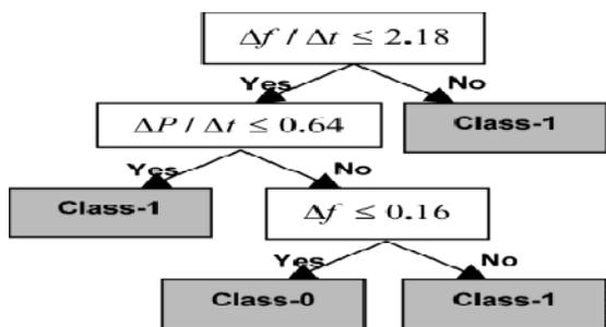
Figure 3 DT-based islanding detection. Class-1 means islanding and class-0 means non islanding
