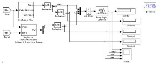
**Figure 2 Fuzzy interference systems for islanding detection**
