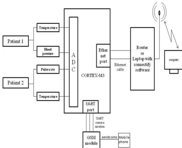
Fig: 2.2.1 Block diagram
