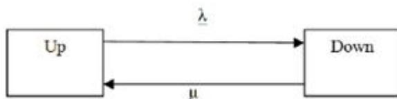
Figure 3 Two State Model for a single component
