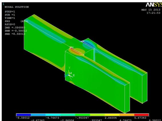
Fig.14 Interlaminar shear stress in  $\tau_{zx}$  direction
