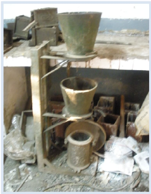
Fig – 3 Compaction Factor Test
