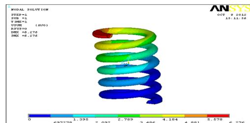
Figure.6: Vonmises stress Displacement results of Carbon Epoxy
