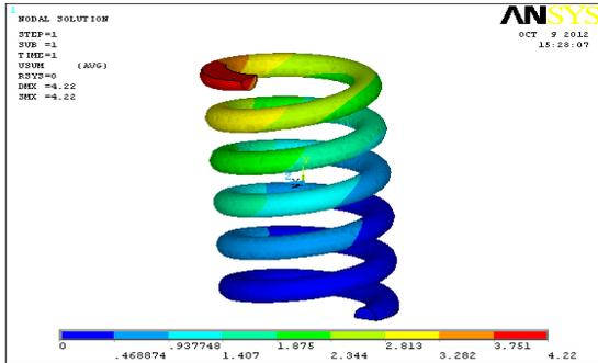
Figure.2: Displacement results of stainless steel wire material
