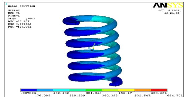
Figure.5: Vonmises stress
