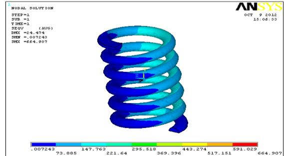
Figure.9: Vonmises stress
