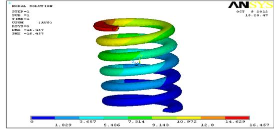
Figure.4: Displacement results of stainless steel wire material
