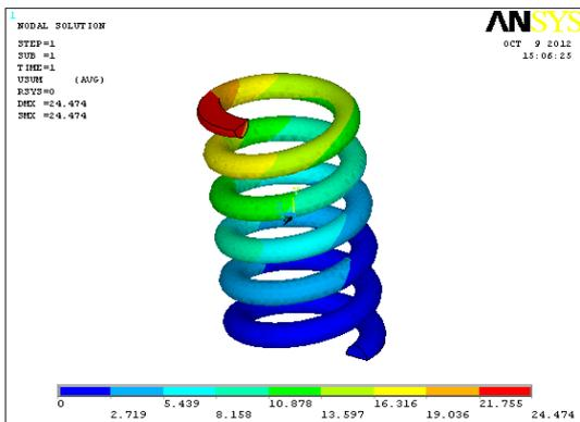
Figure.8: Displacement results of Carbon Epoxy
