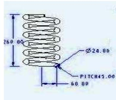
Figure.1: Dimensions of spring
