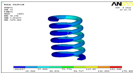
Figure.7: Vonmises stress
