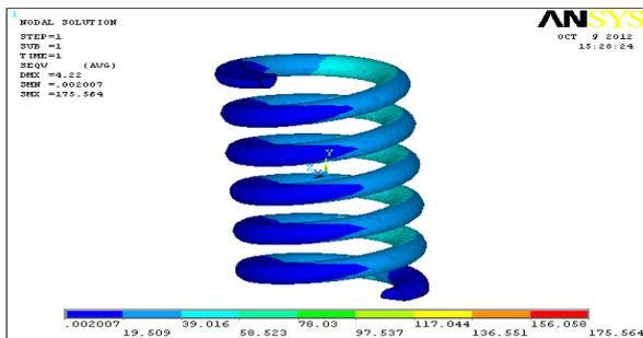
Figure.3: Vonmises stress
