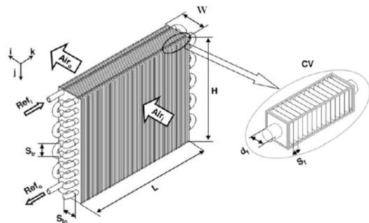
Figure 5: Schematic representation of the heat exchanger discretization. [7]
