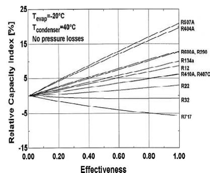
Figure 1: Effectiveness of LSHX vs. Relative capacity index for different refrigerants.[1]
