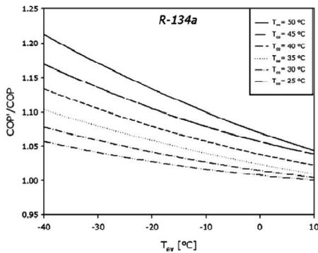
Figure 3B: The COP'/COP ratio for R-134a, for various condensing temperature and evaporating temperature [4]
