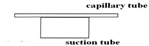
Figure 4A: lateral capillary tube LSHX [6]
