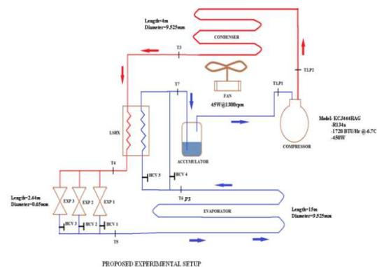
Figure 8: Proposed experimental setup
