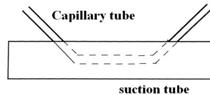
Figure 4B: concentric capillary tube LSHX [6]
