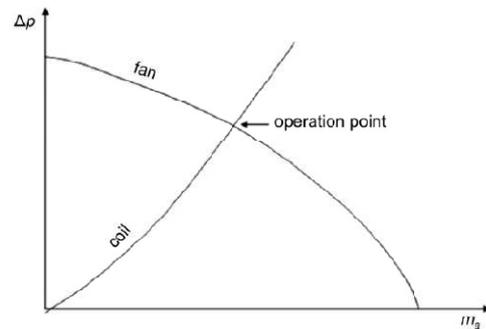
Figure 7: Schematic representation of the fan-coil hydrodynamic interaction [7]
