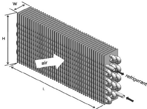
Figure 6: Tube-fin type condenser [7]
