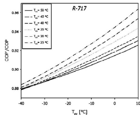
Figure 3A: The COP'/COP ratio for R-717, for various condensing temperature and evaporating temperature [4]
