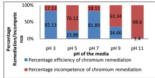
**Fig. 4 Graph of percentage remediation of Cr at different pH.**
