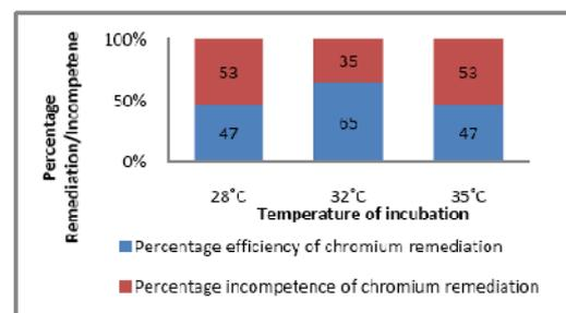
**Fig. 5 Graph of percentage of Cr remediation at different temperature.**
