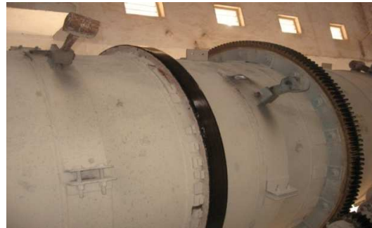
Photograph 1. Showing position of hammer on Rotating drum with 10 rpm speed
