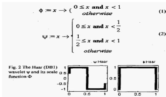
Fig.2 The Haar wavelet and its scale function  $\Phi$
