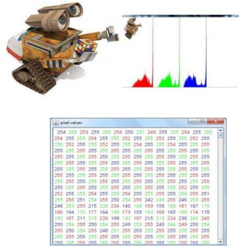
Fig.1 A colored image , corresponding histogram for red green and blue components , and the corresponding pixel values.
