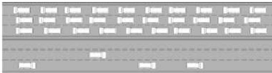
**Fig. 1.** Highway scenario with a traffic jam in one direction of driving and free flow conditions in the other direction. This example represents a typical traffic situation in which congestion control and awareness control protocols might be needed.
