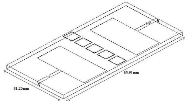
Figure 3. Microstrip Antenna Array with SNG Split Ring Resonators
