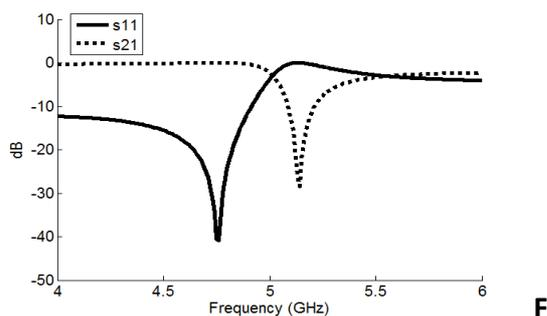
Figure 4. S parameters S11 and S21 for the SNG structure
