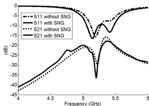
**Figure 8. S parameters S11 and S21 for the array with and without SNG**
