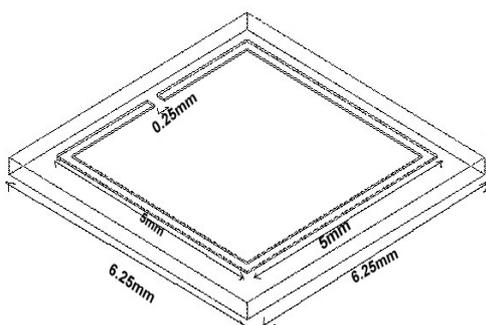
Figure 2. SNG Metamaterial Unit Cell Structure
