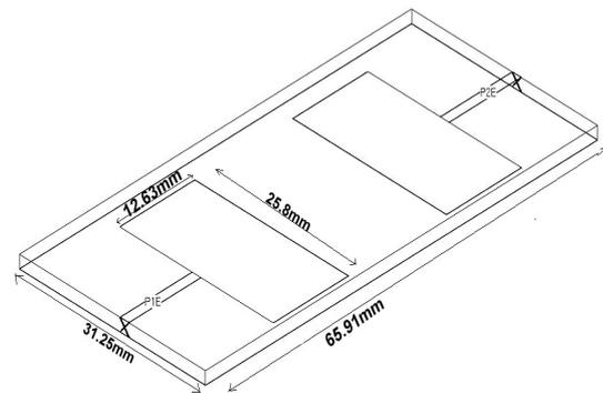
Figure 1. Two element Microstrip Antenna Array Structure
