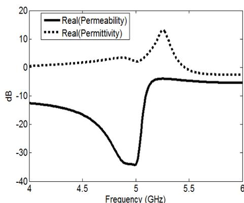
Figure 5. Real part of  $\mu$  (permeability) and  $\epsilon$  (permittivity) for the SNG structure
