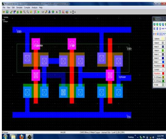
Figure 4. Layout of Phase Detector
