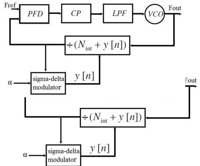
**Figure 2. Block Diagram of PLL using Sigma-delta fractional –N frequency synthesizer**
