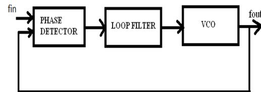
Figure 1. Block Diagram of PLL
