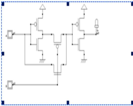
Figure 3. CMOS circuit of Phase Detector
