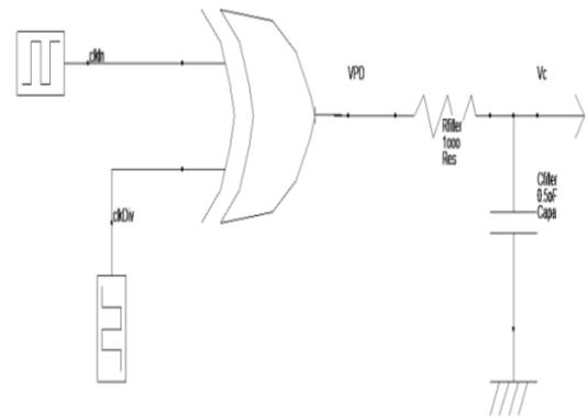
Figure 6. CMOS circuit of Filter
