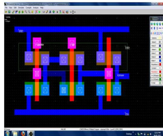
Figure 7. Layout of Loop filter
