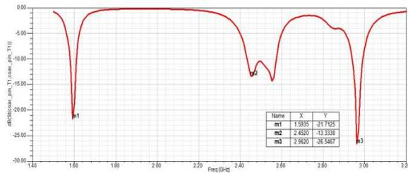
**Fig. 4: Simulated Return Loss for E shape array Antenna**
