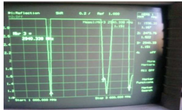
Fig.10. VSWR of Fabricated E-Shape Array Antenna
