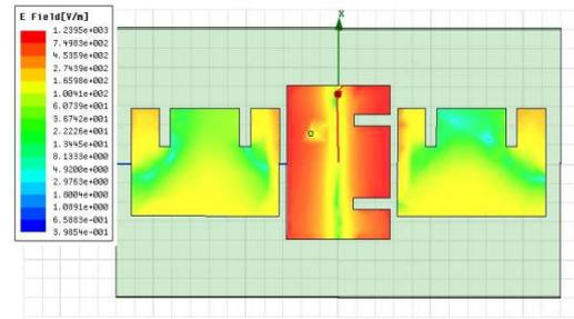
Fig. 8: E-field distribution of E shape array Antenna
