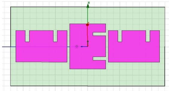
**Fig. 2: E shape array Antenna in HFSS**
