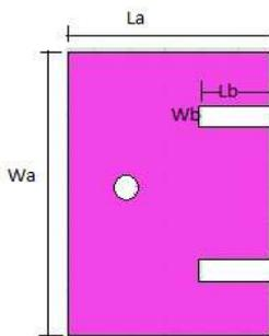
**Fig.1. Design geometry of E shape patch antenna**
