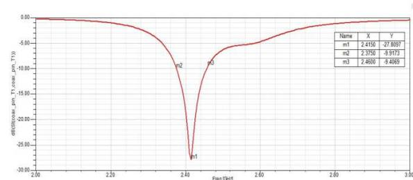
**Fig. 3: Return Loss for the single E shape Antenna**
