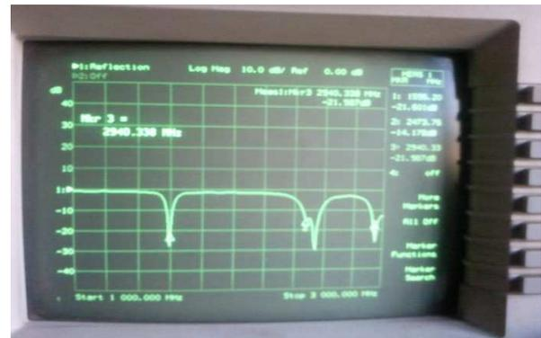
Fig.10. Return Loss of Fabricated E-Shape Array Antenna
