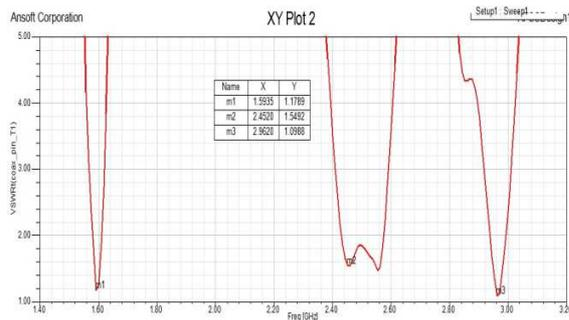
**Fig. 5: Simulated VSWR for E shape array Antenna**
