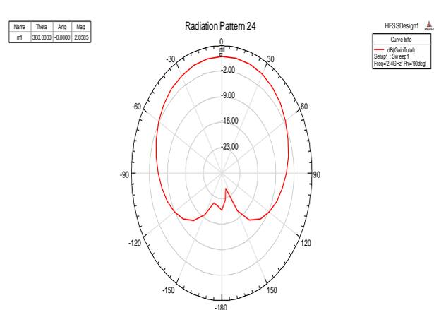
**Fig. 6: Gain of E shape array Antenna**
