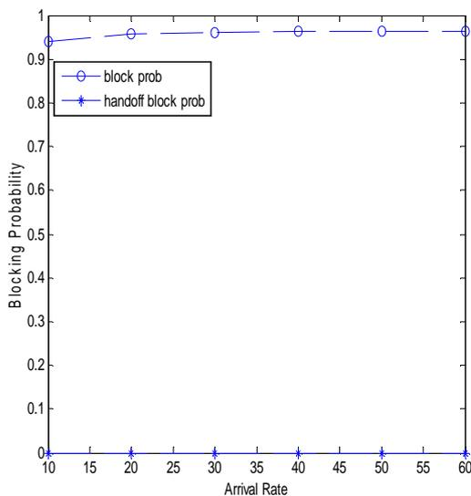
Figure 3: Showing the comparison between new call blocking probability and handoff call dropping during Traffic load
