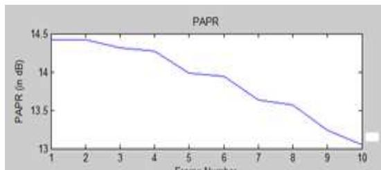
Plot against frame number and PAPR with coding using Rayleigh channel.
