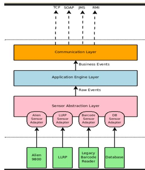
FIG.1 DATAFLOW THROUGH THE THREE ARCHITECTURAL LAYERS
