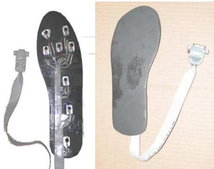
Fig.[5] Transducer placement & design
