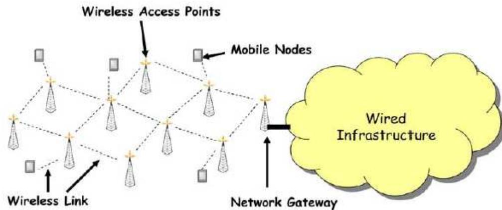
Figure1: Wireless Mesh Network Components: Mobile Nodes, Wireless Link, Wireless Access Points and Network Gateway [2]
