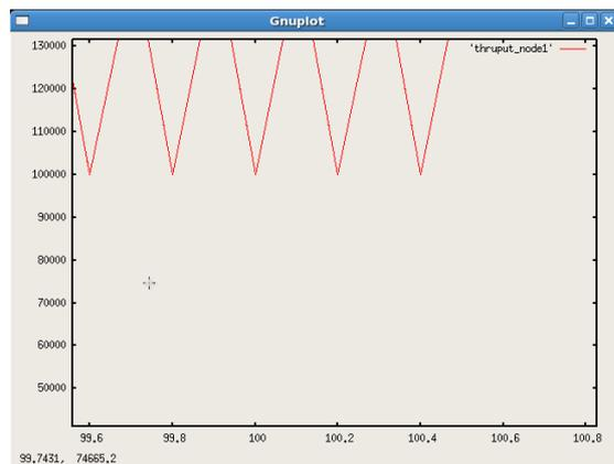
(Figure3: Drop In Throughput for flow 1 to 2)
