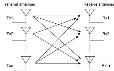
Fig. 1 General block diagram of MIMO
