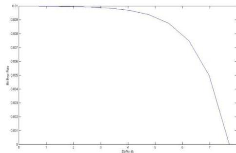
Fig.(b) BER versus Eb/No db plot of 2\*2 MIMO
