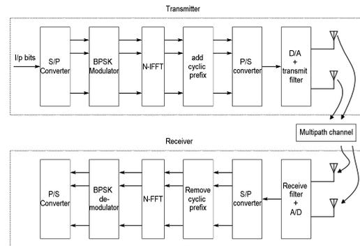
Fig.2 Block diagram of 2\*2 MIMO-OFDM
