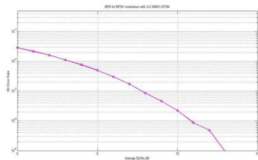
Fig.(c) BER versus Eb/No plot of 2\*2 MIMO-OFDM
