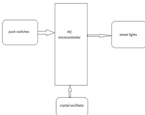
Figure 1: Block Diagram
