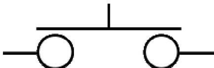
**Figure 9:** Push-to-make switch electronic symbol
