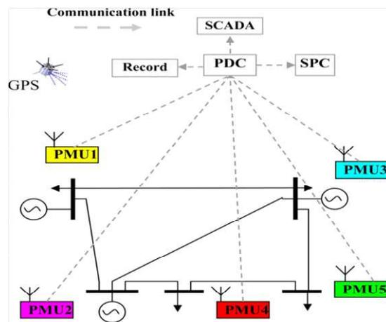
Fig. 3. PMU arrangement at five bus system
