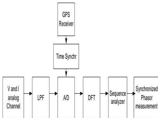
Fig.1. Phasor measurement unit block diagram
