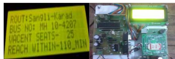
Fig 10: interfacing of Bus stop unit
