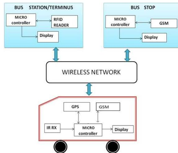
Fig 7: Block diagram of overall system
