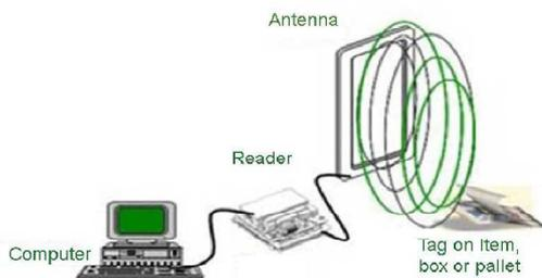
Fig 6: RFID basic operation
