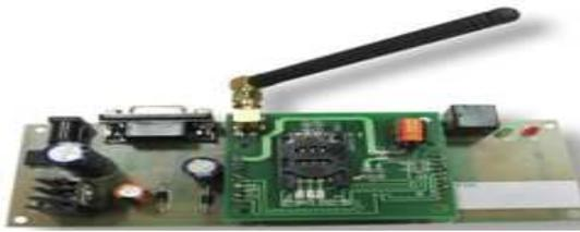
Fig. 2: GSM Modem
