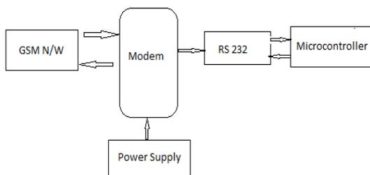
Fig 3: Block diagram of GSM interfacing
