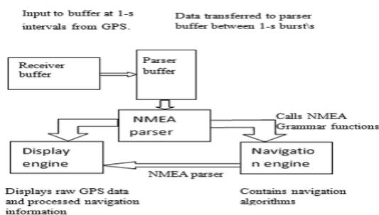
Fig 4: The simple navigation system architecture
