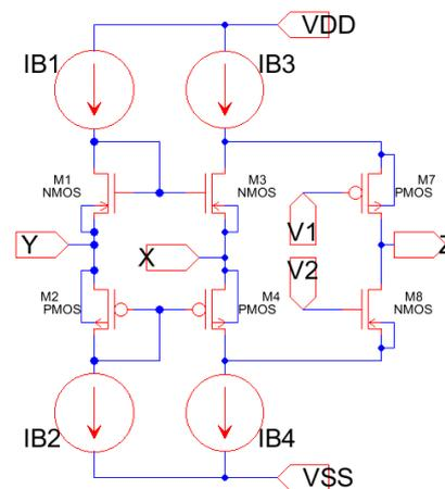
Fig. 4. Schematic of CCII-
