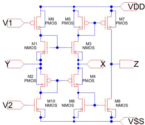
Fig. 3. Schematic of CCII+
