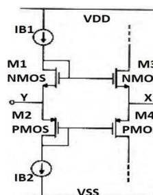
Fig. 2. CCII± input voltage follower stage
