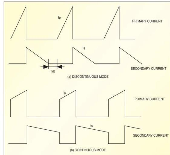
Figure 2: Primary and secondary currents in (a) discontinuous and (b) continuous mode
