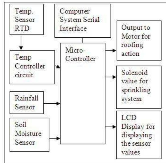
Figure 3: Block Diagram for Irrigation System
