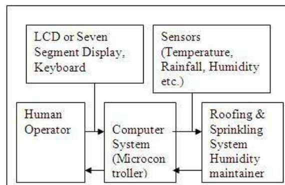
Figure 1 : A Real Time system Model for Irrigation
