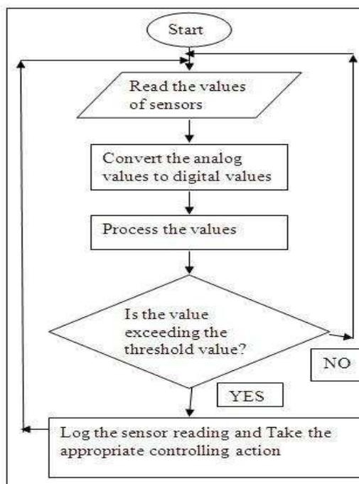
Figure 6 : Flow diagram of the system
