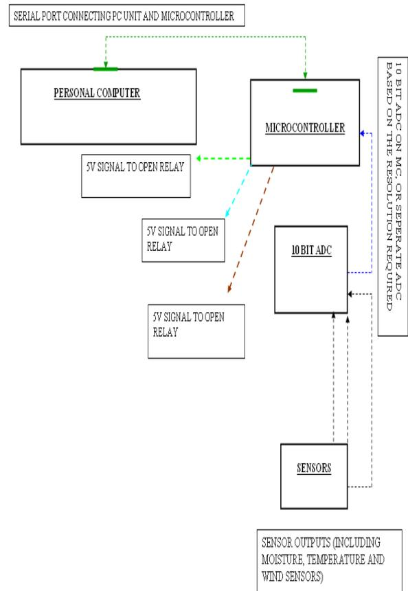
Figure 4: Block diagram of the Smart Sprinkler System
