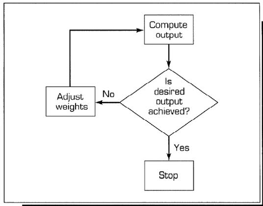
Figure(1): Neural Net block diagram
