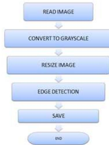
Figure(3):flowchart showing feature extraction of hand gesture images.
