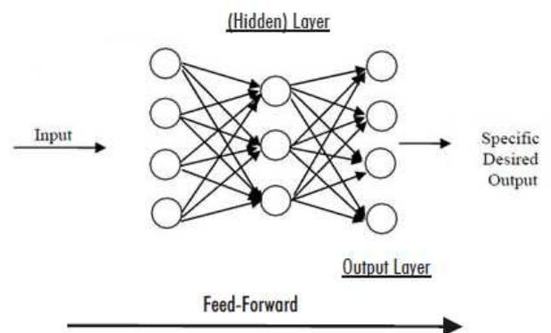
Figure(2):feed forward neural network architecture
