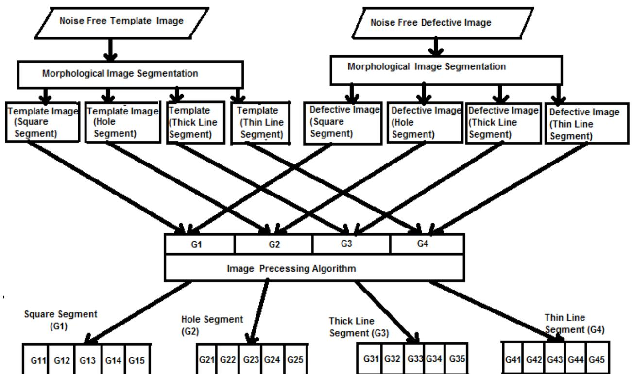
Fig 2. Algorithm for PCB defect classification
