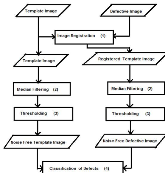
Fig 1. Flow chart of the improved PCB inspection system defined as the process of finding a transformation that aligns one image to another. In this research, geometric transformation is used to find a transformation that aligns a template image and a defective image.
