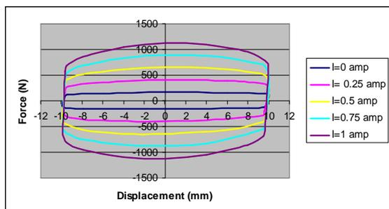
Figure 10(b) .Damping force and displacement curve
