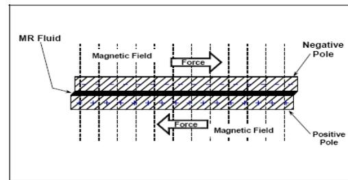
Figure 5 MR fluid in shear mode [14]
