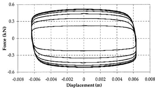
Figure 8(b). Force-Displacement characteristics of MR damper [14]
