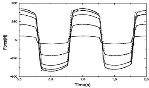
Figure 8(a). Force-Time characteristics of MR damper [14]
