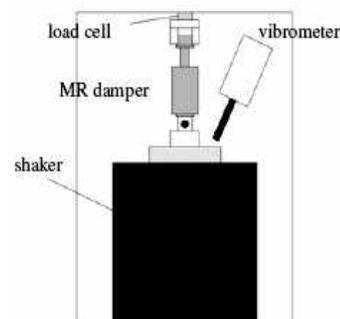
Figure 9 Schematic test setup for the MR damper
