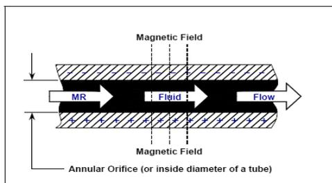
Figure 4 MR fluid valve mode [14]
