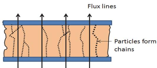
Figure 3 Particles aligning along the flux lines
