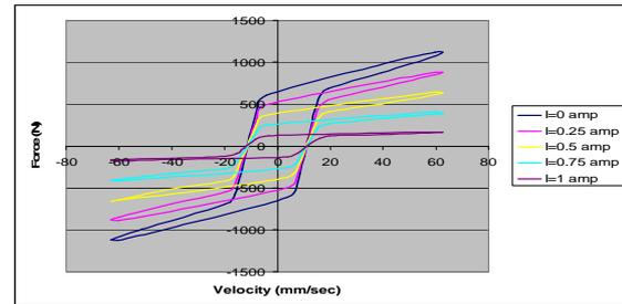
Figure 10(c) Damping force and velocity curve
