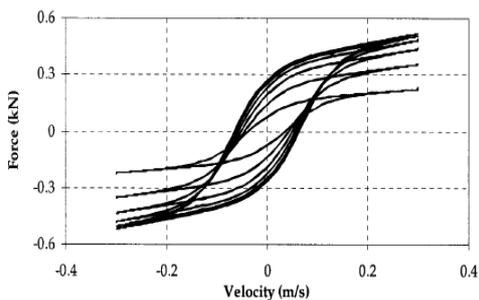
Figure 8(c) Force-Velocity characteristics of MR damper [14]
