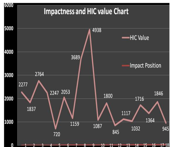
Fig. 6 Evaluation of the friendliness of the original bonnet structure with the pedestrian head
