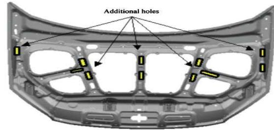
Fig. 1 Pedestrian protection by the modified original reinforcement structure [6]
