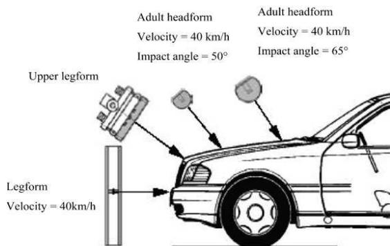
Fig. 2 Pedestrian protection concept proposed by the EEVC WG17 [9]
