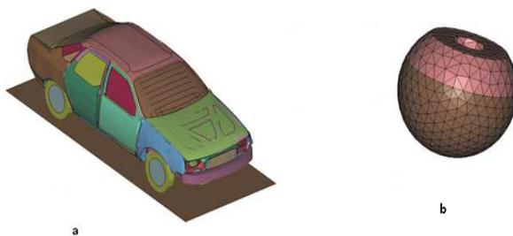
Fig.4 The FE model used in pedestrian – head –bonnet impact simulations: (a) the passenger car model [11]; (b) the headform impactor model [10]
