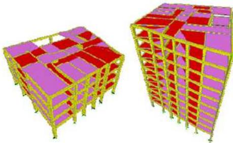
Fig.5.-3-D view of four storey and ten storey building created in SAP-2000.
