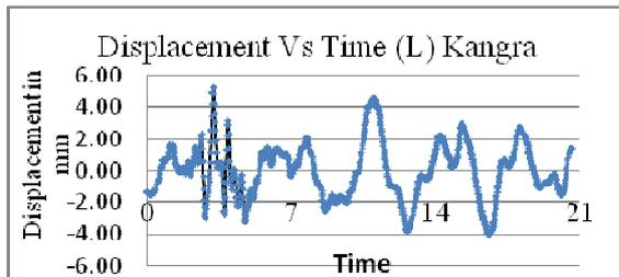
Fig: Displacement time history of top floor (shorter direction) – model 1.
