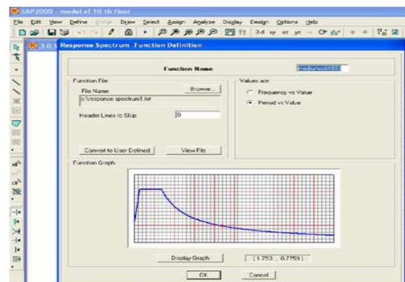
Fig.6- Defining response spectrum function ( $S_a/g$ ) Vs. Period in SAP2000.
