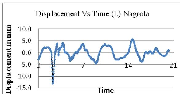
Fig: Displacement time history of top floor (shorter direction) – model 2
