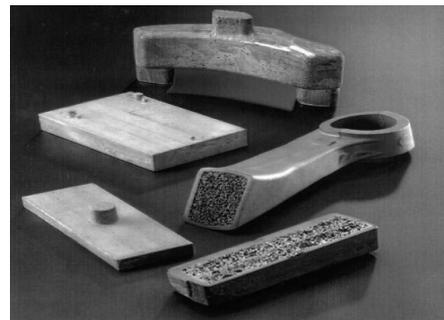
Figure 9: Aluminium castings accomplished with *Permanent aluminium foam core*
