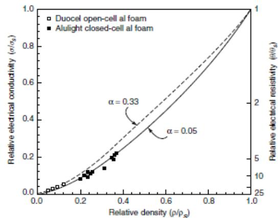
Figure 13: The electrical conductivity and resistivity of open cell and closed cell aluminium foam of different relative density.
