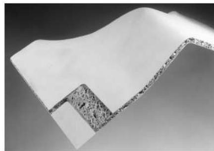
Figure 4: Aluminium foam sandwich
