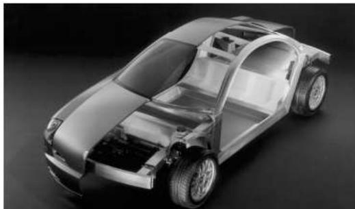
Figure 5. Aluminium Foam Body
