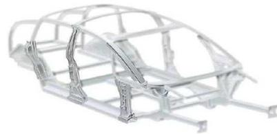
Figure 6: Aluminium spare frame made of hydrofoamed and Welded profiles
