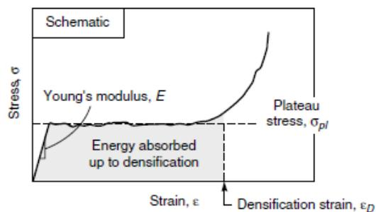
Figure 10: compression stress-strain Curve for aluminium foam
