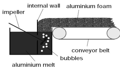
Figure1 - Foaming Melts by Gas Injection
