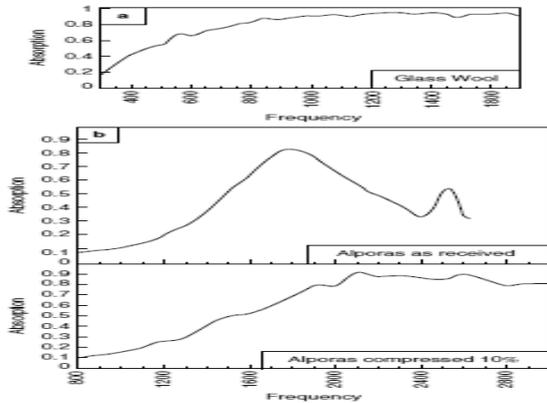
Figure 14. Sound absorption, measured in a plane-wave
