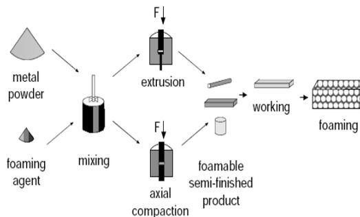
Figure3. Foaming from powder compact process
