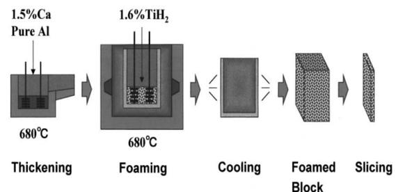
Figure2 Foaming Melts with Blowing Agents
