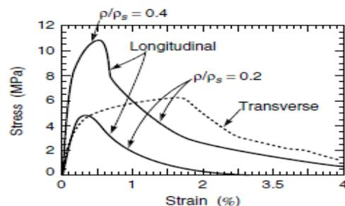
Figure 11: compression stress-strain curve for aluminium foam
