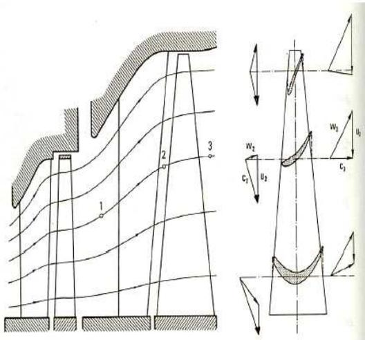
are identical the change in cross section throughout the passage might different task of the designer to find optimum Blade design, nowadays assessed by means of CFD Advanced aft-loaded profiles have streamlines over the blade with varying cross section been designed that make the passage loading more uniform and produce a smaller pressure difference at the leading edge between the concave side and the convex side of the blades. This result in reduced secondary flow losses at blade hub and tip.
