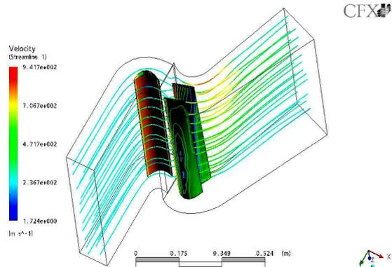
Fig 7.12 Velocity distribution for Untwisted Blade
