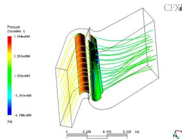
**Fig 7.9 Pressure Streamlines along the flow domain**
