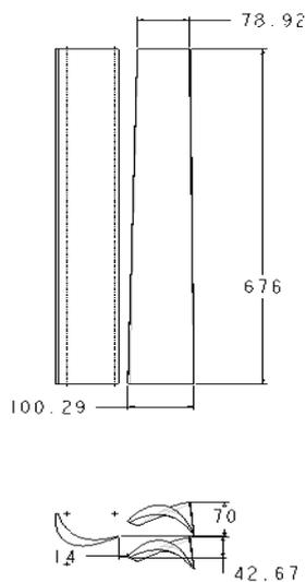
**Fig Blade Geometry**
