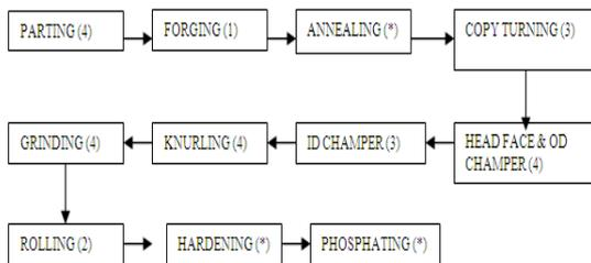
**Fig 1: Manufacturing of Bolts**
