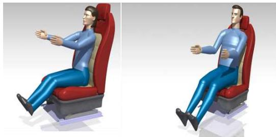
Figure 3.2 Human models testing on conceptual seat in CAD software
