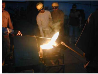
Figure 1.4: Poring of Molten metal into centrifugal casting machine.
