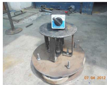
Figure 2.4 Front View of Lock Plate with magnet for attachment and deattachment of plate into machine new design.
