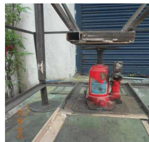
Figure 2.5 Hydraulic jack position below top frame
