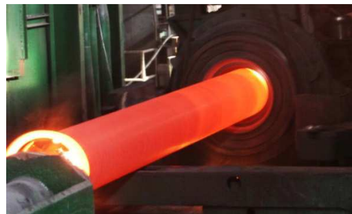
Figure 1.5: Extraction of pipe from machine.
