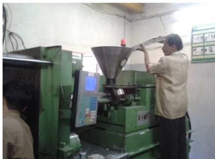
Fig 2. Manual feeding at existing arrangement
