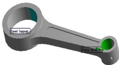
**Fig. 2.4 FEA model of the connecting rod with axial compressive load at the piston pin end and crank end restrained.**
