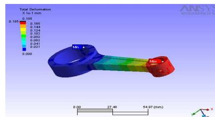
**Fig. 2.8 Total Deformation.**
