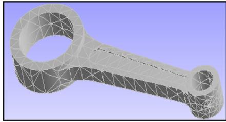
**Fig. 2.3 Meshed Model of Connecting Rod.**
