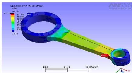
**Fig. 2.5 Equivalent (Von-Mises) Stress.**
