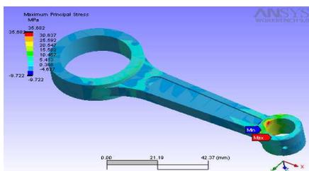
**Fig. 2.6 Maximum Principle Stress**
