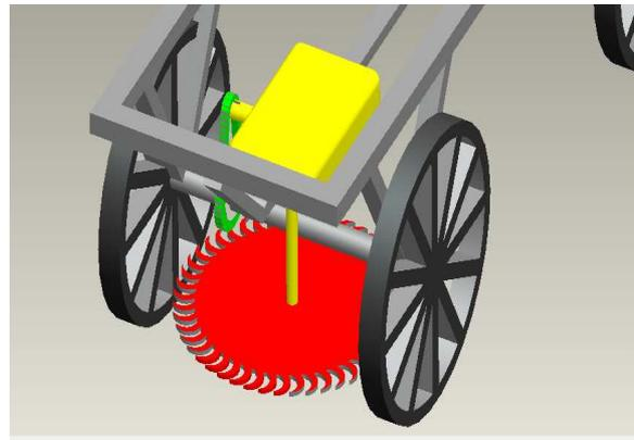
Figure: Cutter and Gear box arrangement.
