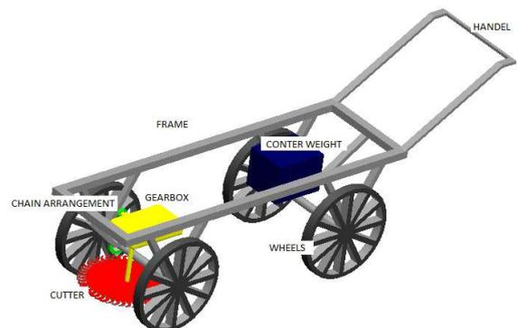
Figure: Conceptual model of wheat cutter for small scale farmer.
