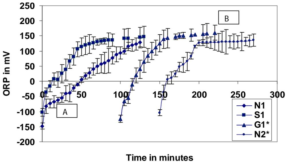
Fig. 2 Aeration of effluents from four field UASBRs: Temporal variation of ORP
