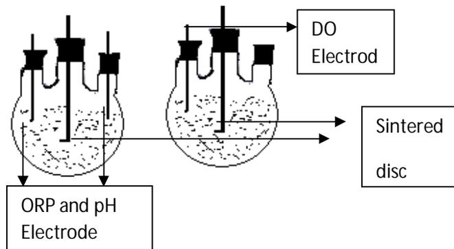
Fig. 1 Schematic presentation of batch reactor
