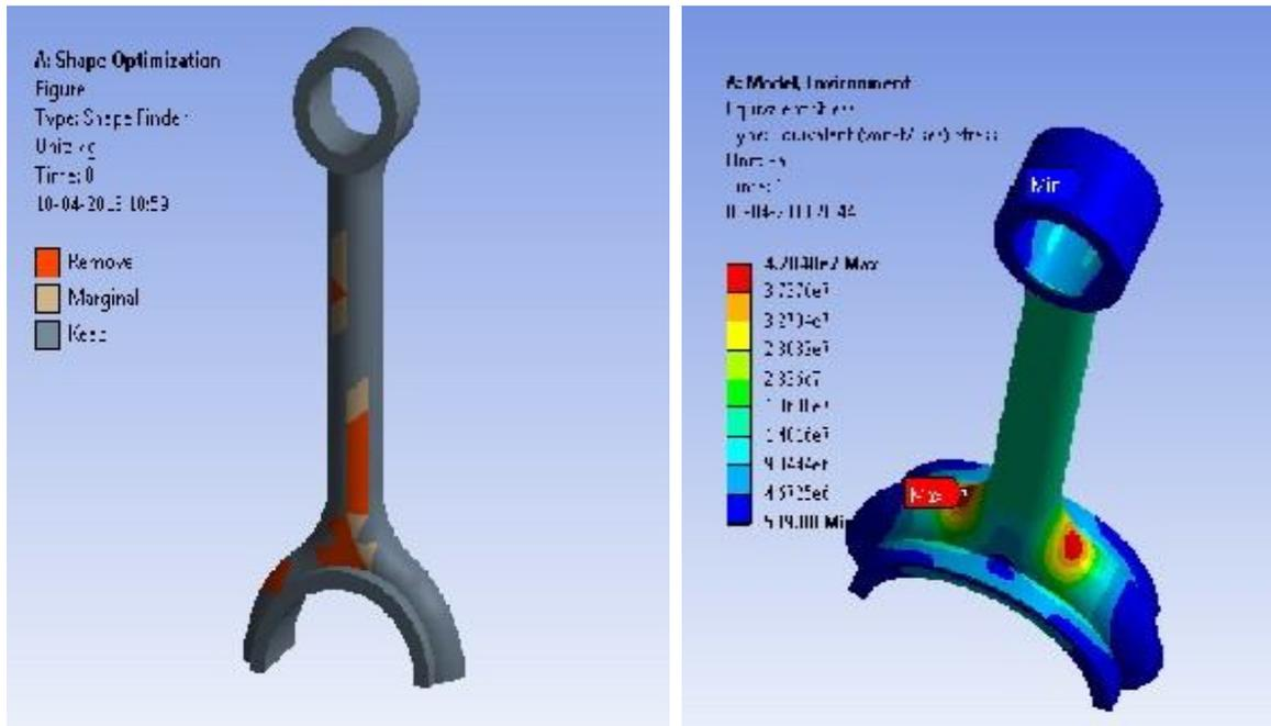
Fig. 1: Equivalent (Von-Mises) stress
