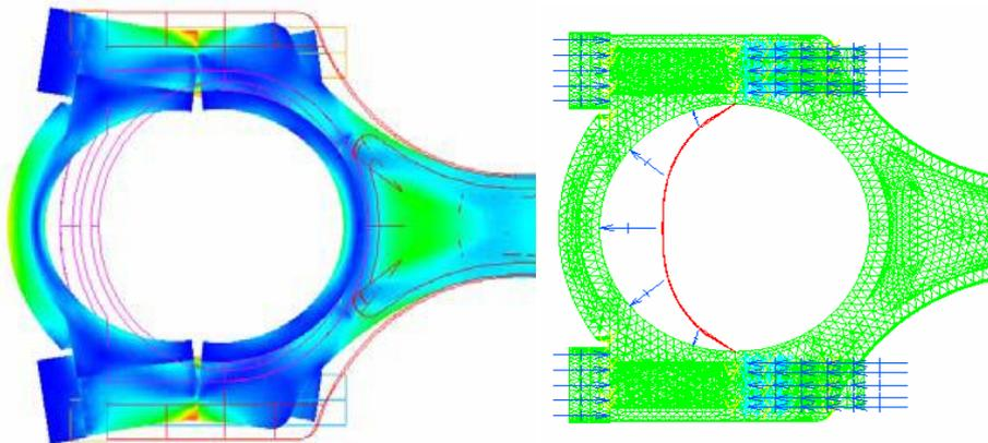
Fig.3: Von Mises stress variation and displacements (magnified 20 times) of the connecting rod and cap under tensile load. The FE model is shown on the right.
