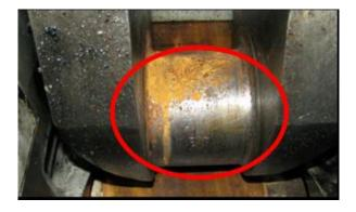
Figure 3.3 Indents in this crank pin journal resulted in this crankshaft being condemned
