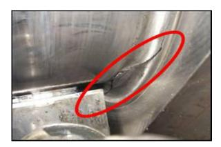
Figure 3.5 Cracking of this crankshaft between the crank pin and the crank web.
