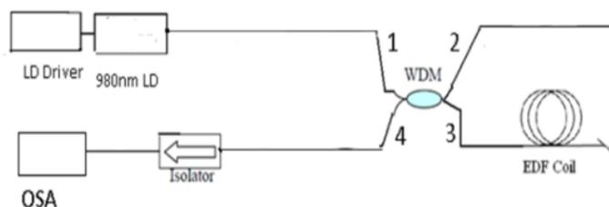
**Fig.5: The experimental setup of SPBS super fluorescent fiber source**
