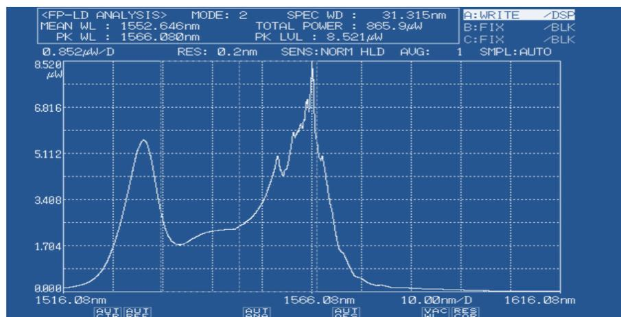
**Fig. 6 The ASE spectrum of SPBS super fluorescent fiber source at 49.08mW input pumps power. Power measured using optical spectral analyses (OSA, ANDO model AQ6317C). The ASE output power is 0.865 mW and the spectral width is 31.315nm.**
