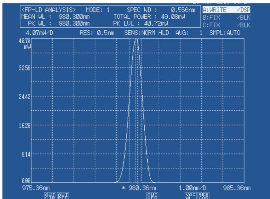
**Fig. 3 Mean wavelength of pump laser diode measured using Optical Spectrum Analyzer (OSA, ANDO model AQ6317C).**
