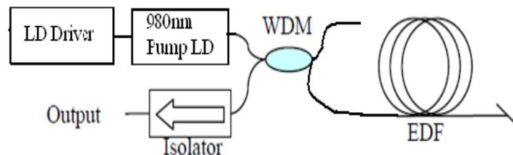
**Fig. 1: Single pass backward signal SFS configuration.**
