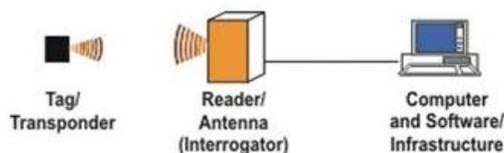
Fig 4: Architecture of RFID system
