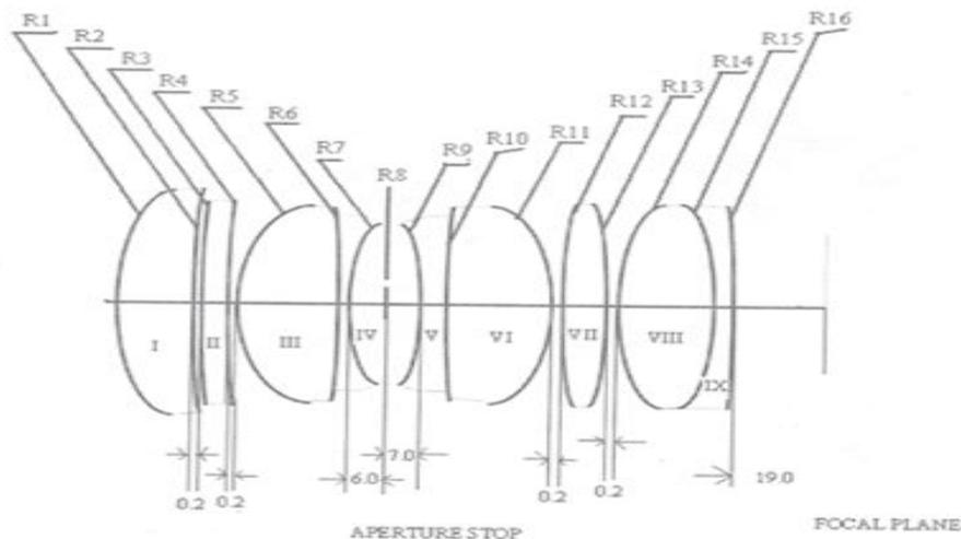
Figure 1: The optical configuration of objective for 25-mm effective diameter opto - electronic image intensifier tube.
